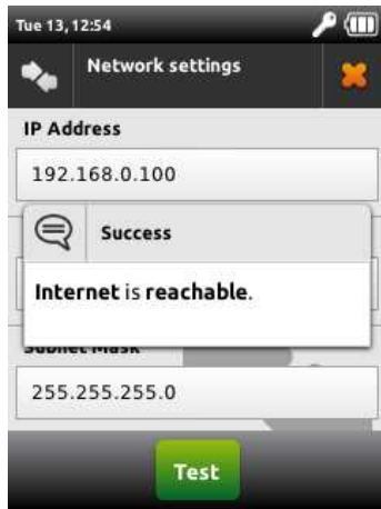
Fig. 18 By pushing the Test button the device will perform a test of connectivity toward the internet.
