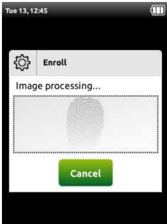
Fig. 5 You have to swipe your finger on the reader several times as prompt, after which the device accounts you into the system.
